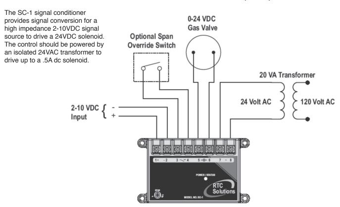
Span Override Switch - When terminals 3 & 4 are shorted together the span setting is ignored forcing the ratio to 100%.
